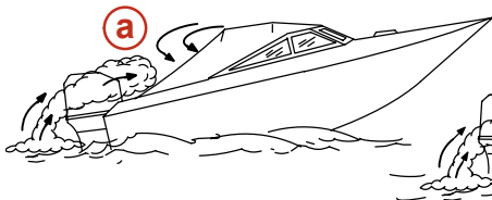
a - Running the boat with the trim angle of the bow too high.
